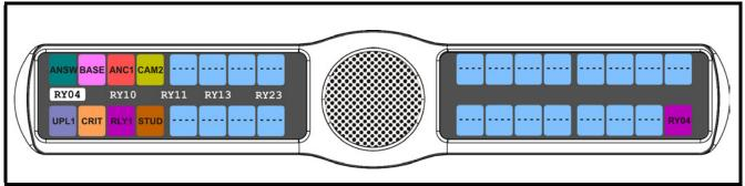
FIGURE 92. Key Assign Menu - System Relay
